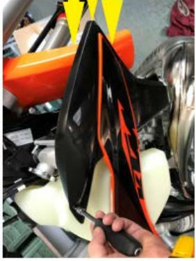
TIGHTEN THE SIDE PLASTIC AND SCREW REMAINING SCREWS ON THE TANK.
