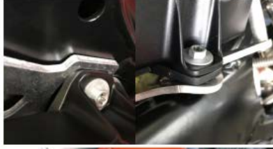
TIGHTEN THE SIDE PLASTIC AND SCREW REMAINING SCREWS ON THE TANK.
