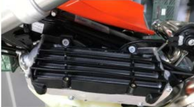
TIGHTEN THE SIDE PLASTIC AND SCREW REMAINING SCREWS ON THE TANK.
